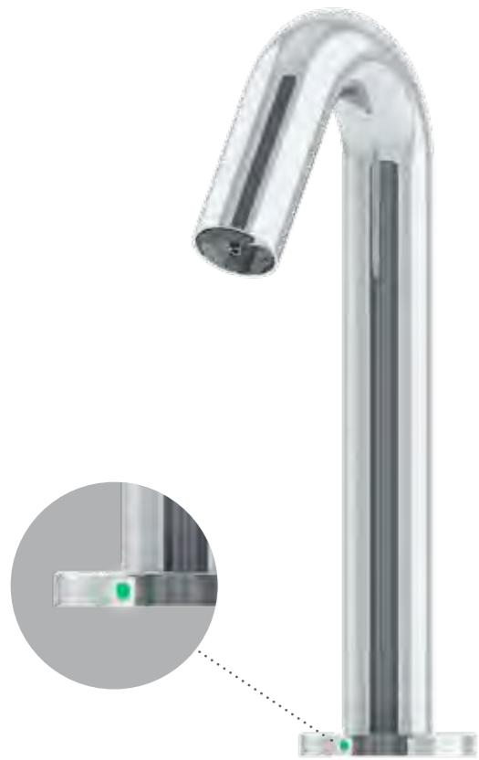
Csaba Soap Dispenser with Soap Level Indicator This new and innovative addition to our popular touchless, automated Csaba line is powered by a 12V transformer and includes a 1.6 Gallon (6L) soap tank suitable for high traffic areas and a level sensor that provides reliable continuous level measurement of soap in the tank. The level indicator is situated in the body of the soap dispenser and shows green when soap tank is full, orange when soap level is low and red when a refill is needed. Other models available. Page 53
